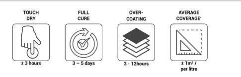
**\*COVERAGE**: The recommended coverage is 1.0 litre per square meter applied in two coats, each with a WFT (Wet Film Thickness) of 500 microns. Each coat will dry to a DFT (Dry Film Thickness) of 275 microns.
